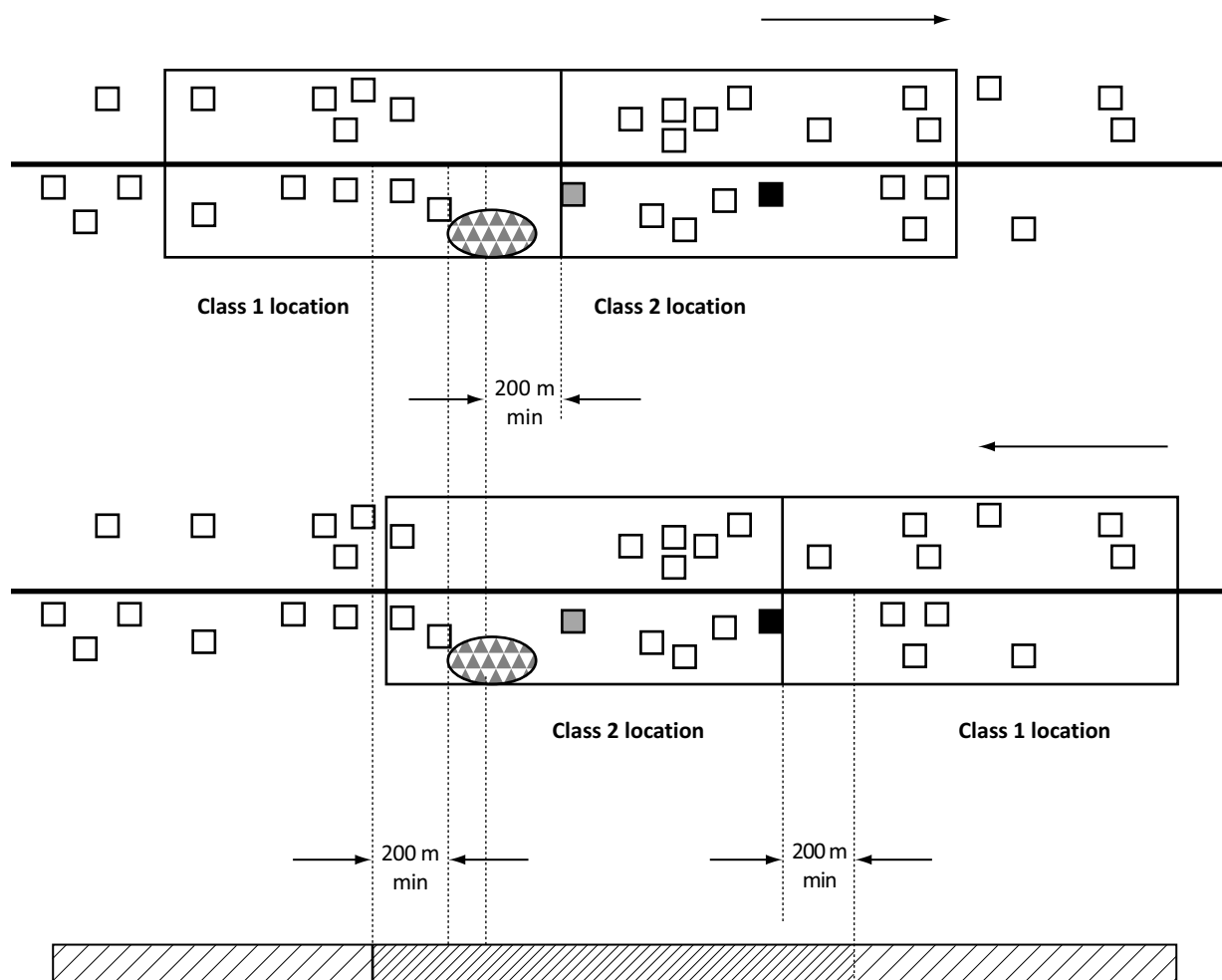
Figure 7 Effect of special feature on end boundary for Class 2 location (See commentary on Clauses 4.3.4.2 and 4.3.4.4 .)
